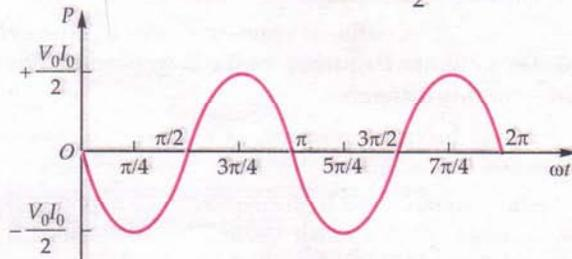
Fig. 7.65 (b) Variation of instantaneous power with  $\omega t$  in an inductive a.c. circuit.
