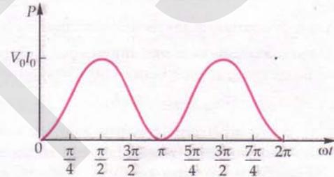
Fig. 7.65 (a) Variation of instantaneous power with  $\omega t$  in a resistive a.c. circuit.
