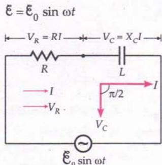
Fig. 7.24 Series LR-circuit.
