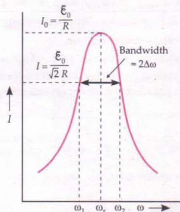
Fig. 7.33 Bandwidth of a series resonant circuit.
