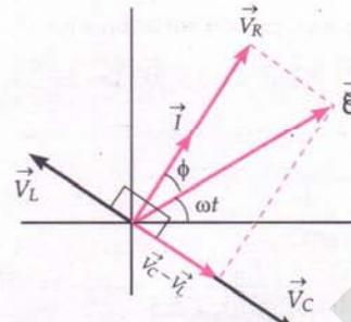
Fig. 7.30 Phasor diagram for a series LCR-circuit when  $V_L < V_C$ .
