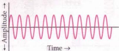
Fig. 7.48 Undamped oscillations.
