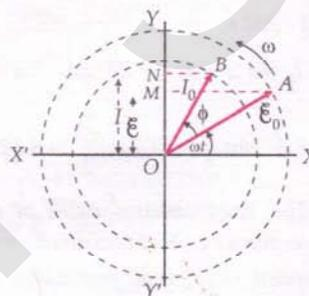
Fig. 7.3 A phasor diagram for an alternating emf and current.
