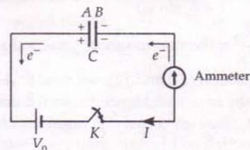
Fig. 7.9 A capacitor in a d.c. circuit.
