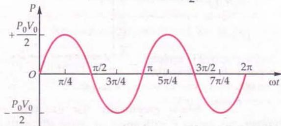
Fig. 7.65 (c) Variation of instantaneous power with  $\omega t$  in a capacitive a.c. circuit.
