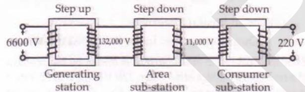
Fig. 7.52 Schematic diagram of a distribution system.
