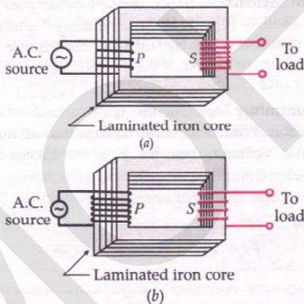
Fig. 7.50 (a) Step-up and (b) step-down, transformer.
