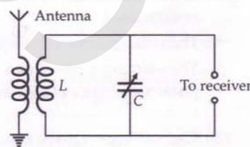
Fig. 7.34 Series resonant circuit.
