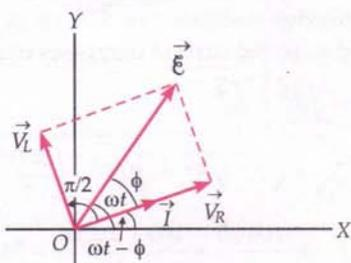
Fig. 7.16 Phasor diagram for series LR-circuit.
