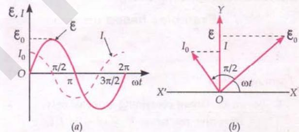
Fig. 7.13 (a) Graph of  $\mathcal{E}$  and  $I$  versus  $\omega t$  and (b) Phasor diagram, for a capacitive a.c. circuit.
