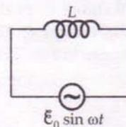
Fig. 7.6 A.C. through an inductor
