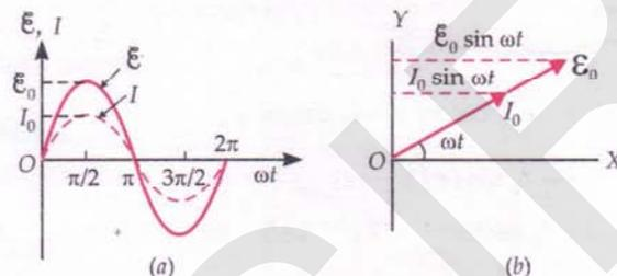
Fig. 7.5 (a) Graph of  $\mathcal{E}$  and  $I$  versus  $\omega t$  and (b) Phasor diagram, for a resistive a.c. circuit.
