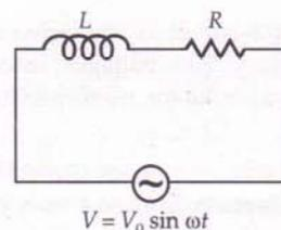
Fig. 7.40 Choke coil.
