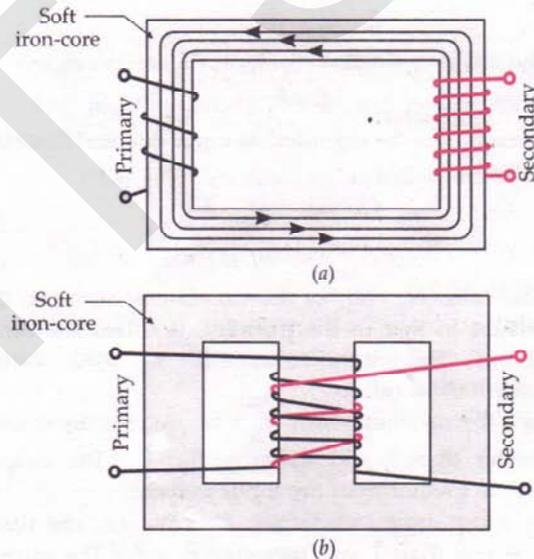
Fig. 7.51 (a) Core type and (b) Shell type transformer.
