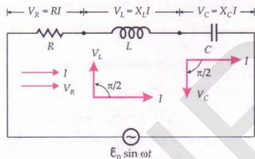
Fig. 7.27 A series LCR-circuit.
