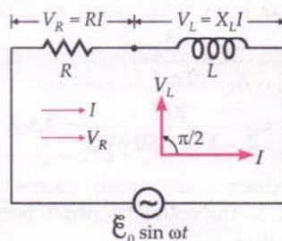
Fig. 7.15 A series LR-circuit.
