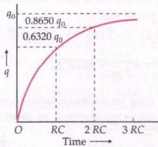
Fig. 7.10 Variation of charge  $q$  with time  $t$  during the charging of a capacitor
