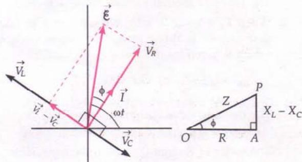
Fig. 7.28 Phasor diagram for a series LCR-circuit when  $V_L > V_C$ .
