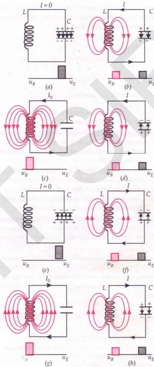
Fig. 7.47 The oscillations in an LC-circuit.
